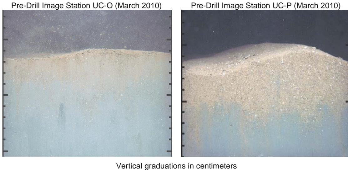
Physical processes appear to dominate the seabed surface at the stations in the study area. Biogenic activity of benthic organisms is limited to a few burrows and voids that appear to be related to feeding activities of subsurface fauna. Prism penetration, a proxy for sediment compaction, correlates to sediment grain-size with lowest penetration, and therefore higher compaction, at fine sand stations and highest penetration (lowest compaction) in fine sand-silt-clay and silt-clay sediments.
