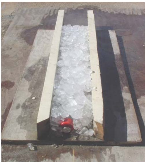
FIGURE 1. A soil core capped and cooling in an ice bath. The thermometer is visible in the end cap.
