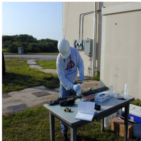
FIGURE 2. A soil sample being collected from along the length of the core into a bottle containing methanol.
